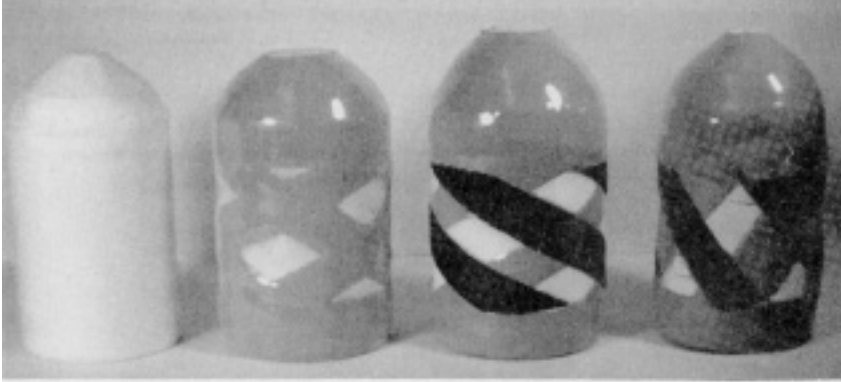
FIGURE 5.79 Plastic pig designs.
